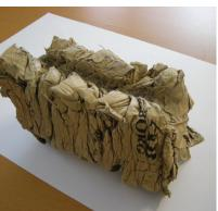
**DESIGNED FOR CARDBOARD COMPACTION** The model Brickman 300 Cardboard is ideal for compaction of dry cardboard and paper. The compaction pressure is up to 500 kg/cm<sup>2</sup>.
